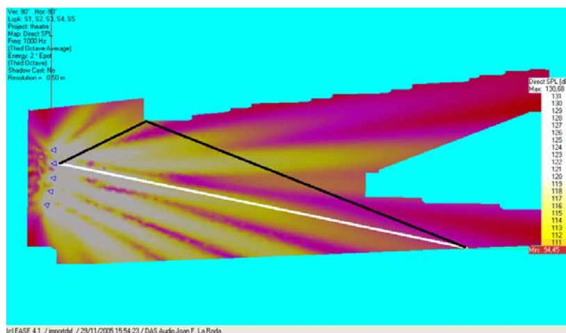
Fig. 1. System with a poor vertical directivity control.
