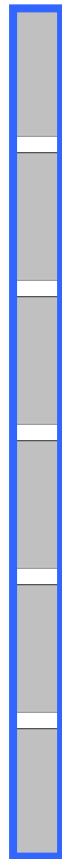
Fig. 14. The sum of discreet rectangular shaped radiating surfaces behaves like one single sound source.
